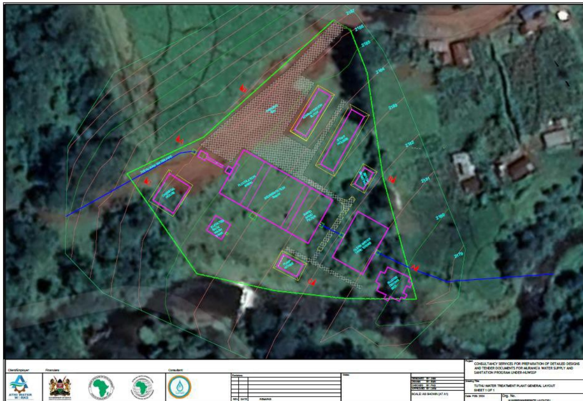
Figure 2-6: :Layout of the Proposed Tuthu Treatment Plant
